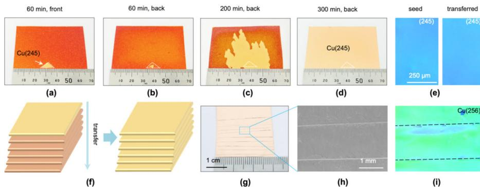
Fig.3-1-39 Replication preparation of single-crystal copper foil with targeted facet
