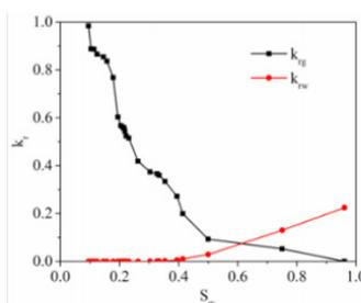
**Calculated shale gas-water relative permeability curve based on pore network model**
