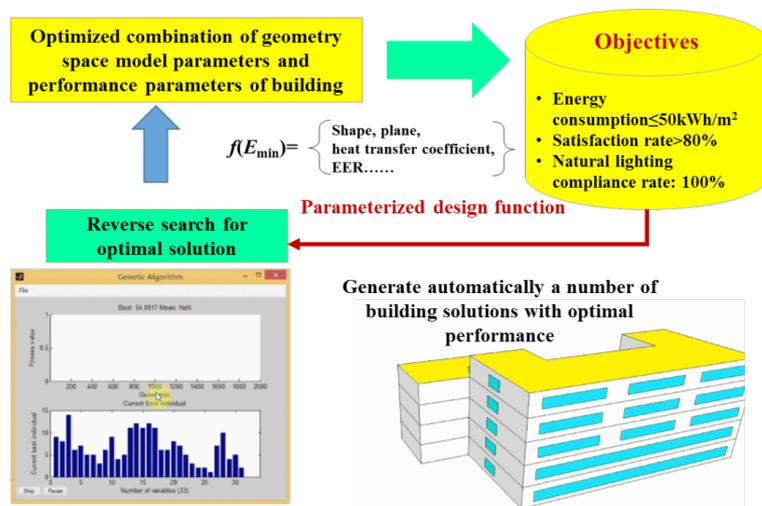
Fig. 3-1-41 Reverse generation method of construction scheme with energy saving as target
