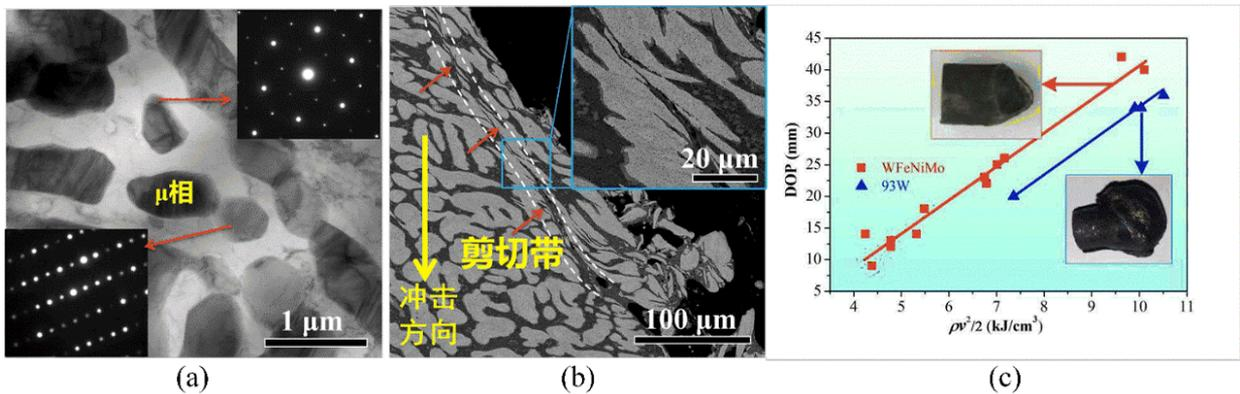
Fig.3-1-4 A new type of tungsten high-entropy alloy with outstanding self-sharpening capability: (a) ultra strong  $\mu$  phase precipitations, (b) shear-banding induced by high strain gradient, (c) this new alloy achieves the 10-20% larger penetration depth than 93W.
