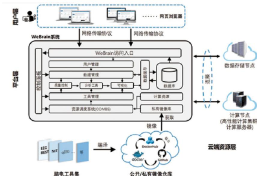
Fig.4-7-4 Based on the cloud-native cloud brain science platform WeBrain, it can realize the integration of tools, data and computing Nodes in the cloud, so as to promote multidisciplinary international cooperative research
