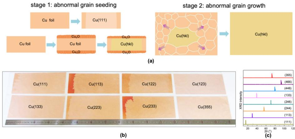
Fig.3-1-38 Preparation of large-size single-crystal copper foil library
