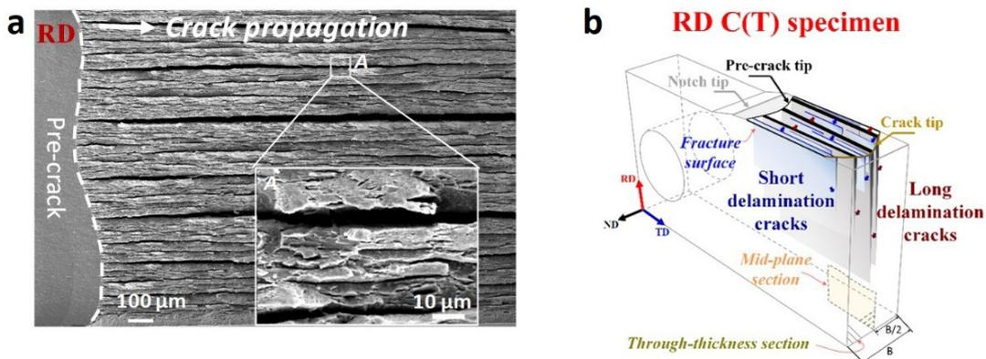
Fig. 3-1-37 The fracture surface and schematic diagram of toughening mechanism of D&P steel. (a) The fracture surface of D&P steel, showing intensive delamination cracks. (b) The schematic diagram of the D&P C(T) specimen, showing the direction of delamination.
