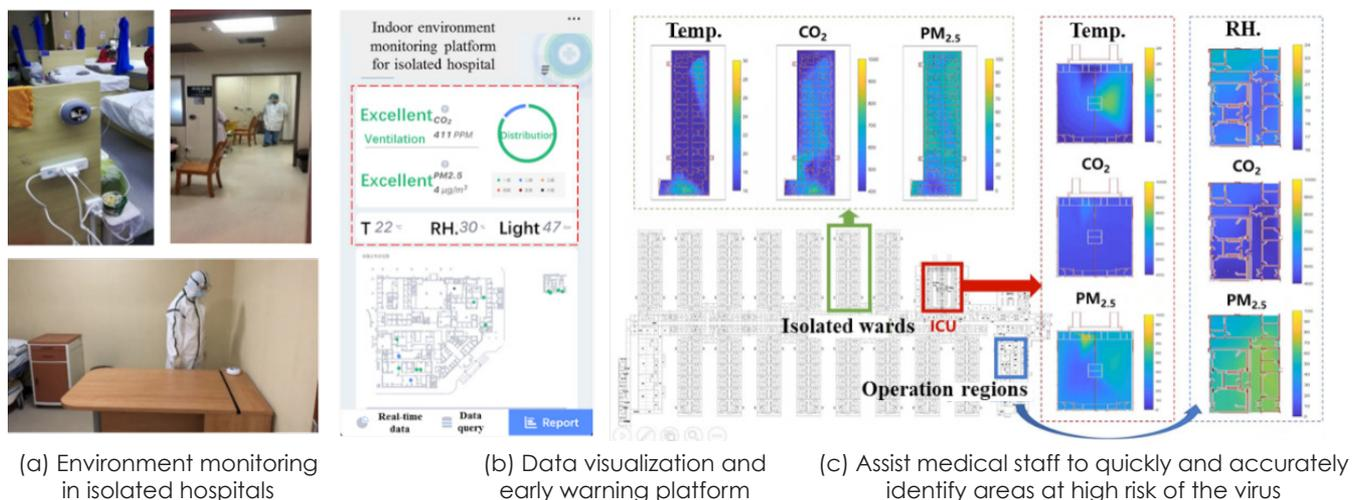
Fig.3-1-42 Real-time warning technology for environmental health risks in buildings and its application in isolated hospitals
