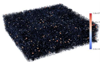
**Shale multi-scale pore network model**
