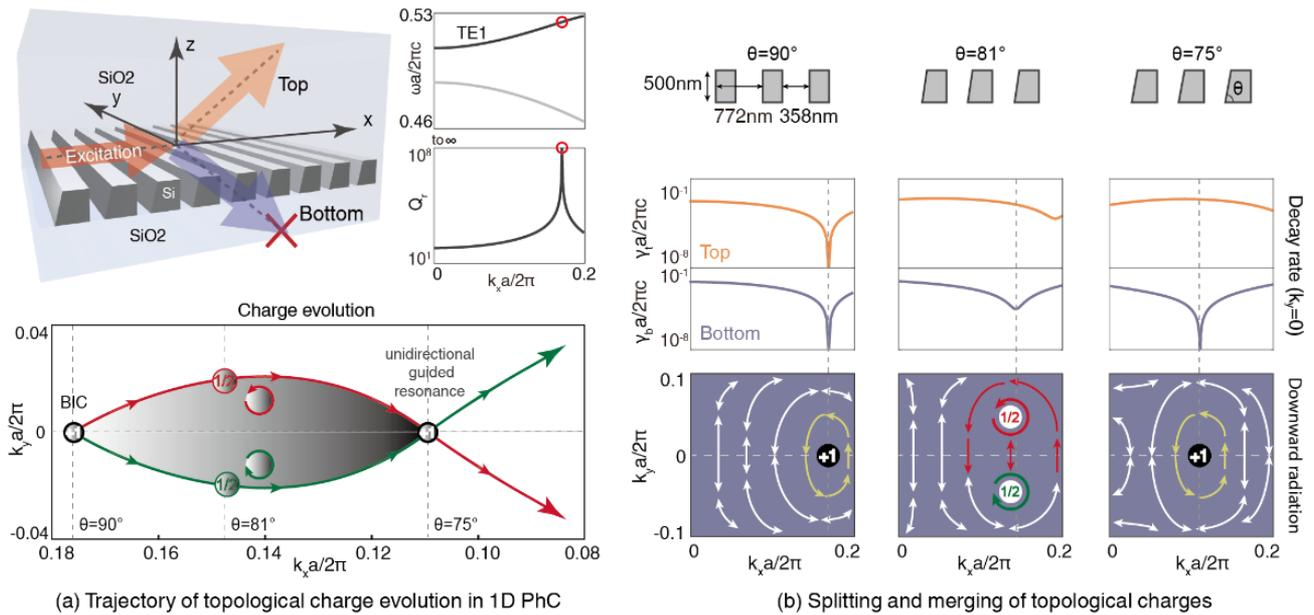
Fig. 3-1-48 Unidirectional guided resonance from manipulating the evolution of topological charges
