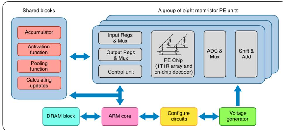
Fig. 3-1-47 System architecture of memristor-based CIM
